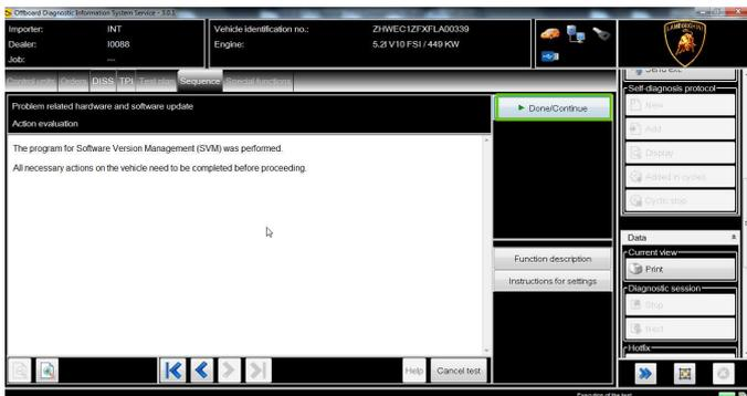
36. Once the update is finished and the SVM program is completed the vehicle has to go in sleep mode.
